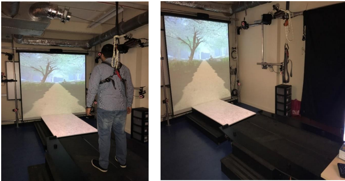
Figure 1 The CAREN System located at National Centre of Prosthetics and Orthotics, University of Strathclyde. The system is an advanced treadmill with integrated motion capture cameras. Furthermore, for safety the system has a harness that can hold the full body weight to prevent any falling.
